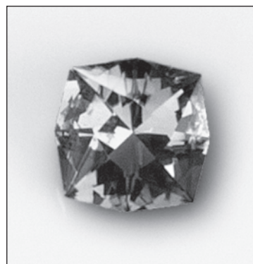
Figure 12-15 A pleochroic tourmaline showing yellow-green colours along the up-down direction and pale blue-green left and right..
