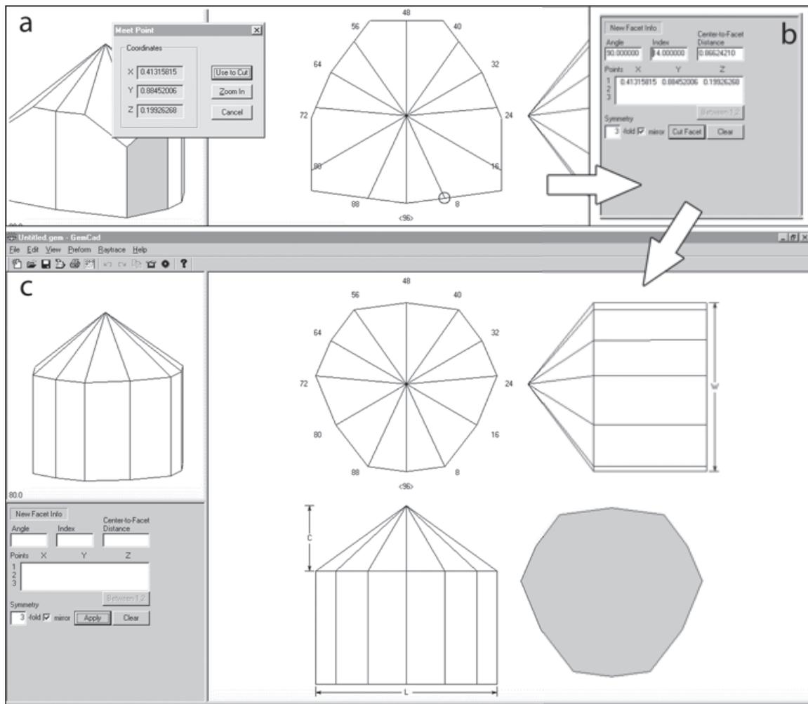
Figure 18-12 Click on the facet intersection to set a meet point (circled at top). Then enter the correct angle and index for the second set of girdle facets (upper right). Clicking on **Cut Facet** finishes the girdle outline (bottom).
