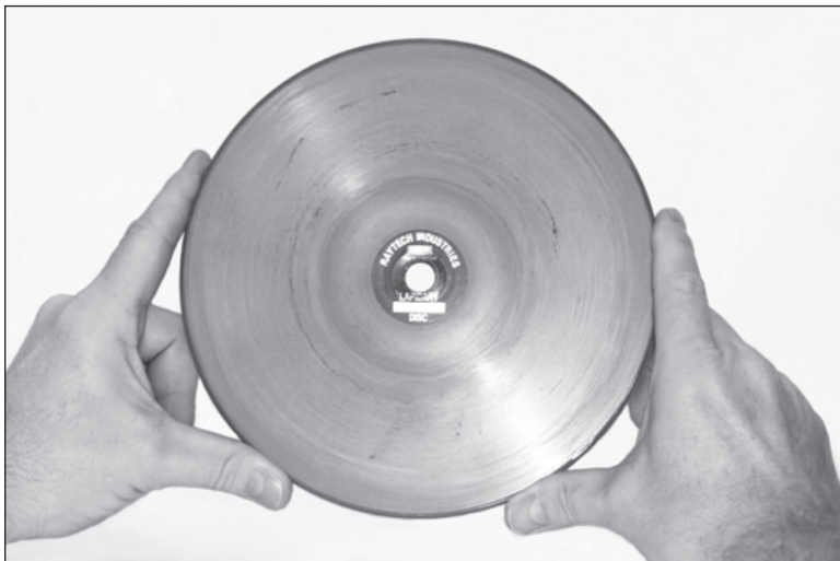
Figure 3-5 The NuBond cutting laps have a composite resin matrix surface layer embedded with diamond.
