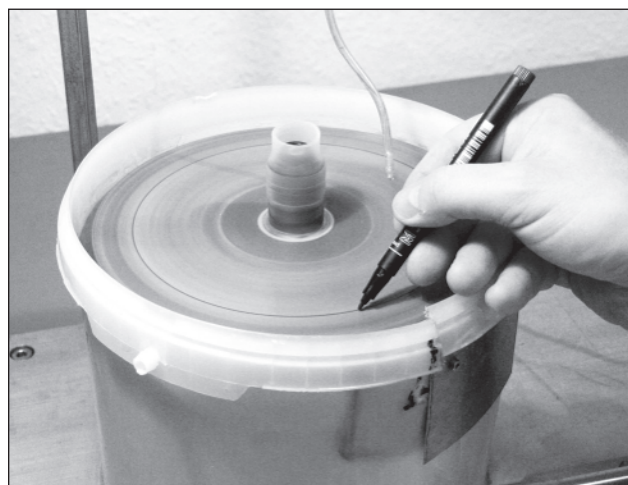
Figure 5-36 Mark the lap with a permanent marker and always test for depth of cut at the same radius.
