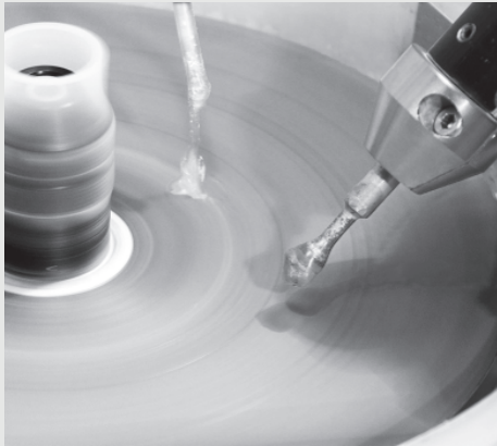
Figure 5-34 Locate the water drip inward of the minimum radius of lap you plan to use, and ensure a steady flow of water to wash away cutting residue and prevent scratching. Wiping a clean finger from inside to outside can help distribute the water.
