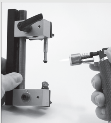
Figure 7-9 Heat a small blob of dop wax.
