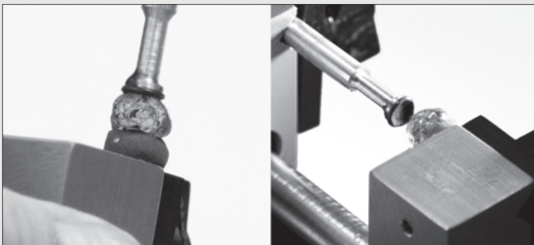
Figure 7-10 Squeeze the stone and dop together briefly to produce a wax impression. This eliminates gaps for dopping with cyanoacrylate glue.
